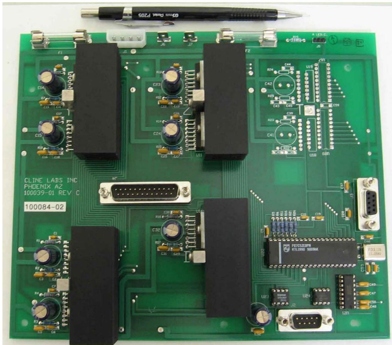
The basic motor driver is pictured below. It has a SUB-D 9 Pin RS232, SUB-D 9 Pin from 6 home switches, SUB-D 25 Pin to three stepper motors and one dc clamp motor, 4 Pin Power connector connects with a 250Watt PC power supply having 12Vdc and 5Vdc inputs.
